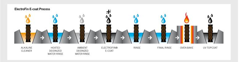
Electrocoating is the process by which a metallic workpiece (coil) is submerged in a paint / water bath where electricity is used to deposit paint onto it. ElectroFin E-coat is a factory-applied corrosion-resistant coil coating which is applied in one of our two e-coat facilities.
