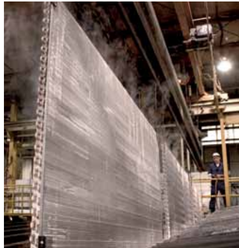
Heated alkaline cleaning process to remove contaminants
